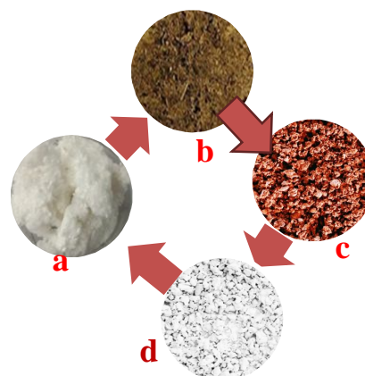
Figure 6: (a) Animal waste, (b) Digested animal waste by Kraft method, (c) Bleached cellulose (d) Isolated cellulose.
