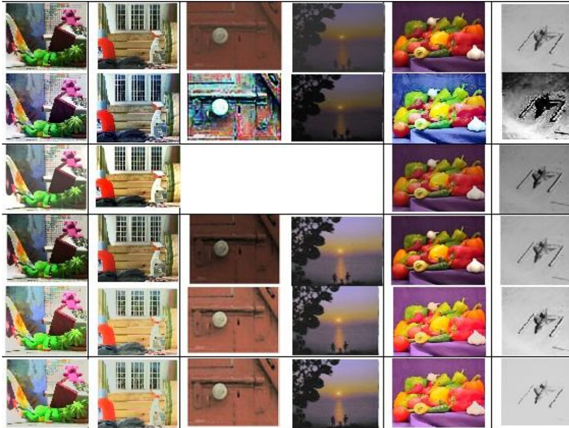
Figure 2: Restored image by different methods (a) Original Image (b) Histogram equalization method(c) Method (d) V-transform method (e) Proposed method. (f) Proposed method with sharp filter.
