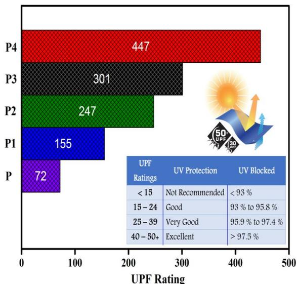
Figure 5: UV shielding properties of PANI/ graphite/ GO/ rGO/ graphene-coated cotton fabric.
