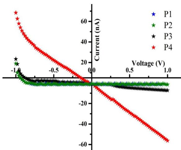
Figure 6: I-V characteristics of the PANI composite coated fabric.
