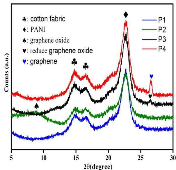
**Figure 4: XRD pattern of PANI/ graphite/ GO/ rGO/ graphene-coated cotton fabri.**
