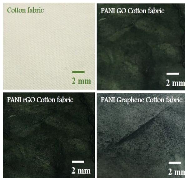
**Figure 2: Photography of bare cotton fabric and PANI/Graphene related coated cotton fabric.**
