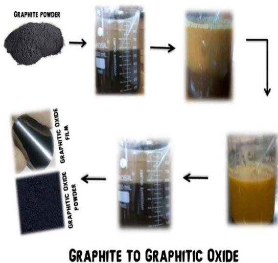
**Figure 1: GO synthesis process by modified Hummers method.**
