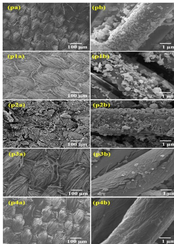
**Figure 3: FESEM observation of (pa,b) PANI-coated CF, (p1a,b) PANI/ Graphite coated CF, (p2a,b) PANI/ GO coated CF, (p3a,b) PANI/ rGO coated CF, and (p4a,b) PANI/ Graphene coated CF.**
