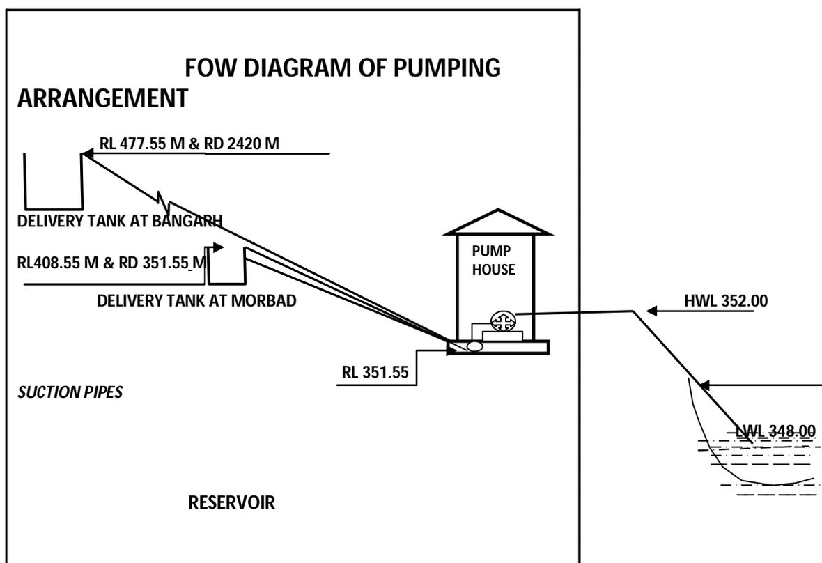
**Figure 2: Flow Diagram of Pumping System.**
