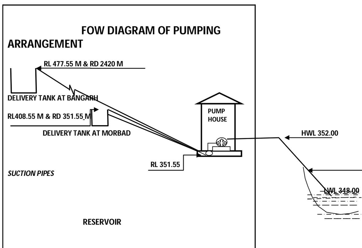
**Figure 2: Flow Diagram of Pumping System.**
