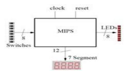
Figure 1: Block diagram.
