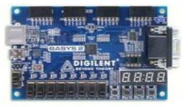
Figure 2: Digilent Basys2 FPGA Board.
